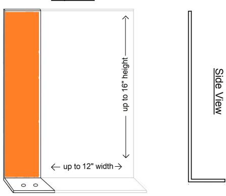
Our Custom Flex Barrier Markers are made of a high impact plastic and are offered in a wide variety of sizes. Making this one of the most versitile barrier delineation products on the market that can meet just about any specification (local, state or federal).
